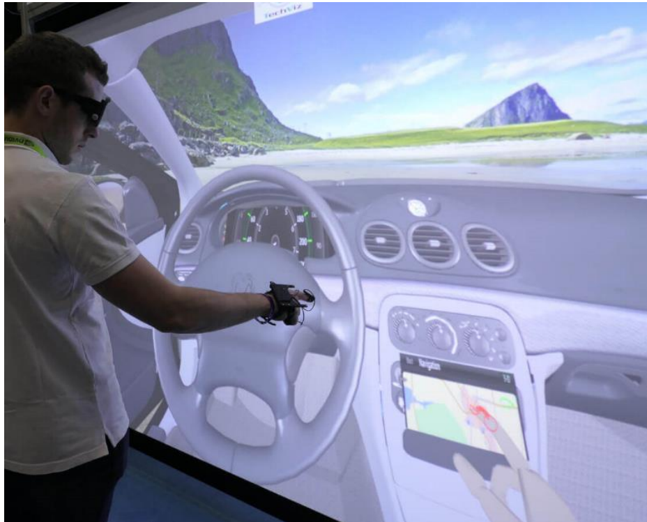
Virtual touchscreen to test HMI
